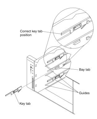
Figure 61. Installing a drive compatibility key
